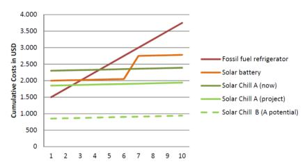
Figure 1:Comparative cumulative costs of conventional and SolarChill refrigerator over lifetime.
