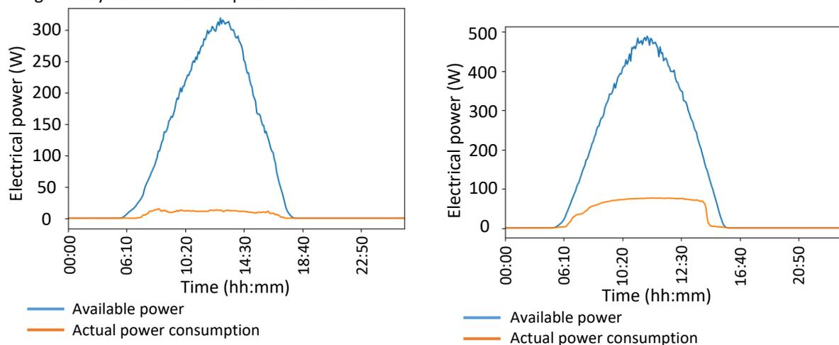
**Figure 6: Available and consumed power over the course of the day, exemplarily shown for a device of type 1 (left) and type 2 (right)**
