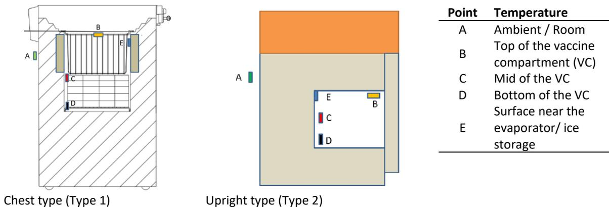
**Figure 3: General position of temperature sensors for the two cabinet types**
