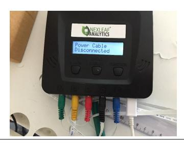
"Power cable disconnected" appears if voltage is too low for charging and is not critical
